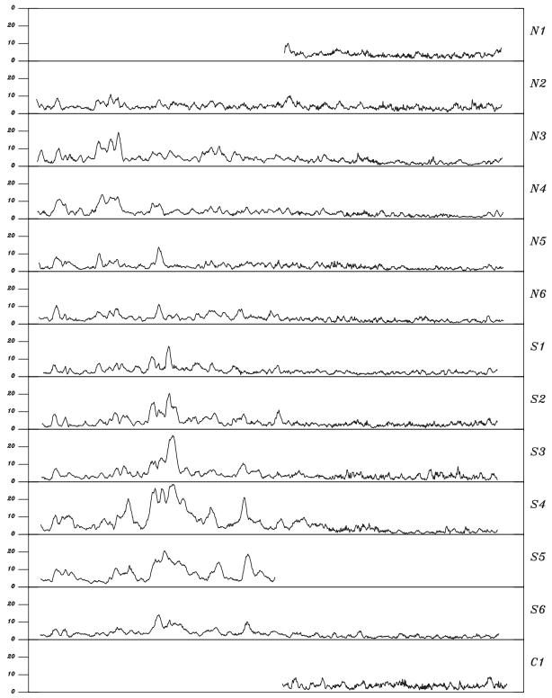
Figure 2. The vertically averaged amplitude of the negative rotary spectra at only 1.10 cpd for the 13 ADCP moorings indicates the main peaks occur in May through September. Very little variability occurs during winter. The variability in the southern line during July and August is correlated to the passage of a typhoon event traveling northeast and passing across Kyushu (see wind stress in Figure 5).
