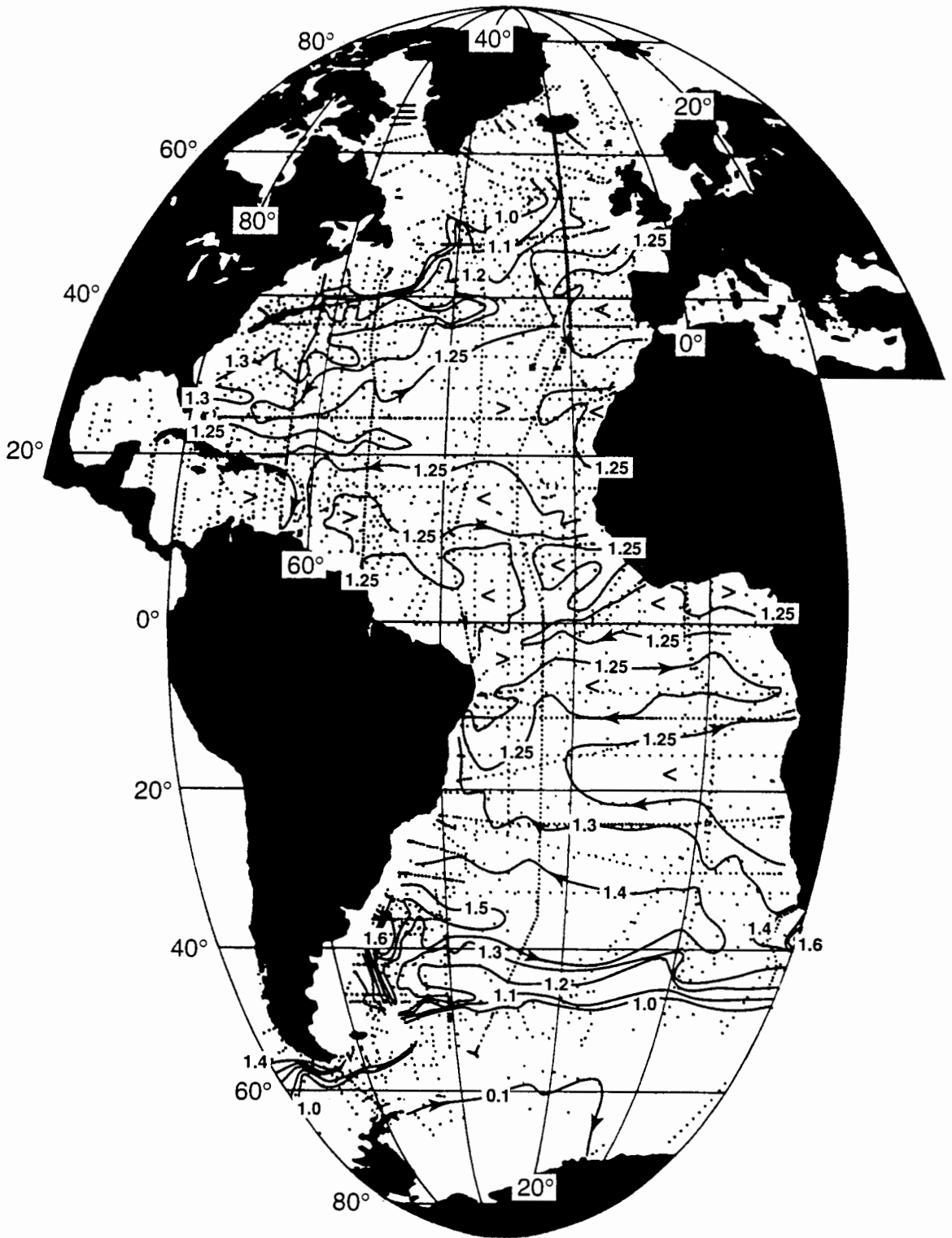
Figure 7. Pressure anomaly streamfunction (dyn m) at 31.7\sigma_{\theta} relative to 3000 dbar. A mean pressure of 750 dbar was subtracted prior to calculation. (Following Zhang and Hogg 1992).
